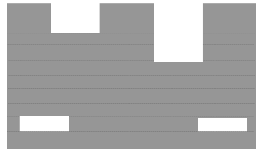
Figure 10. The amount, or possibility, of delamination occurring is dependent on location of air cavity relative to other package structures.
