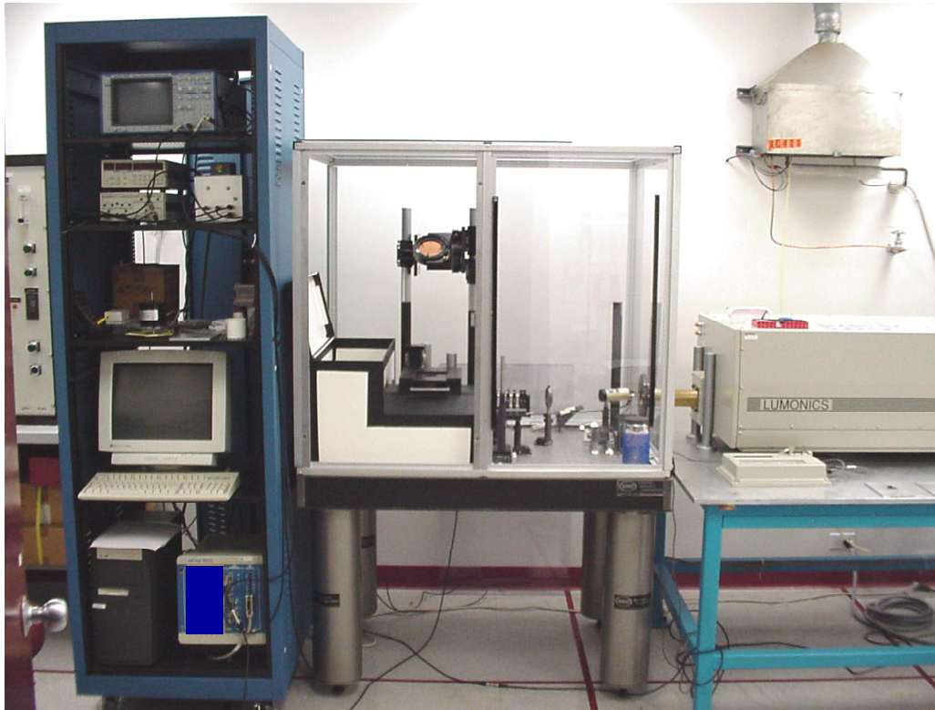
KAI Proprietary TC System used to validate thermal material properties used in package design (1999).
