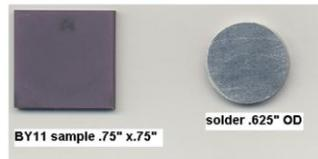
2-1/4 layer alumina sample and cast solder sample. Solder sample checked for internal voiding due to BGA sphere oxidation upon ceramic crucible melting.
