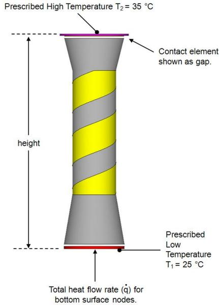
**Fig. 8: CGA Sub-Model Effective Thermal Conductivity Calculation Description.**
