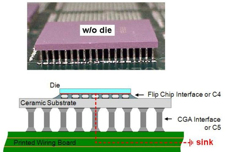
Fig. 1: Assembled Ceramic CGA Package (Top). Package Schematic (Bottom).
