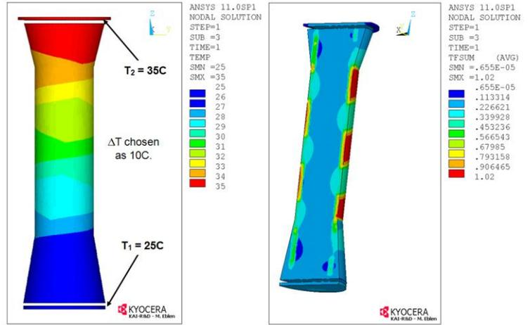
**Fig. 9: Sub-model Results. Temp Plot (left), Thermal Flux Vector Sum Plot (right).**
