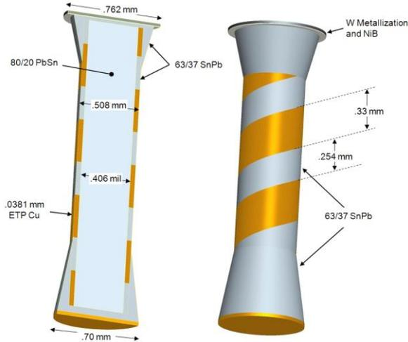
Fig. 5:  $6\sigma$  CGA Interconnect Pro/E Model.
