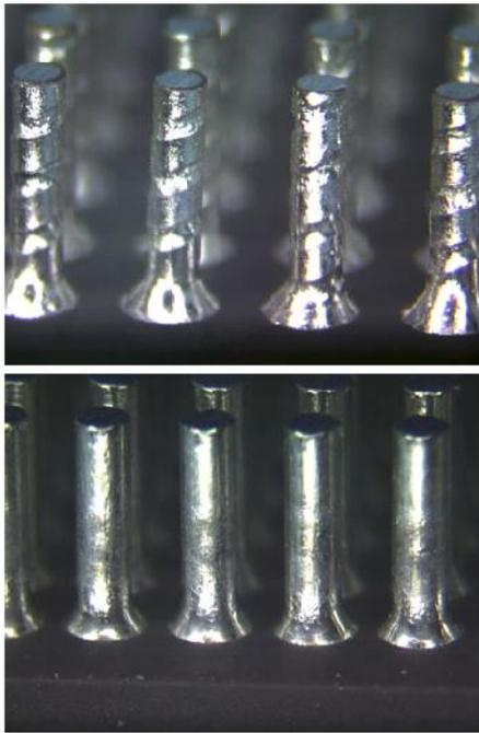
**Fig. 2:  $6\sigma$  CGA (Top). Conventional IBM Style CLASP CGA (Bottom). [2]**
