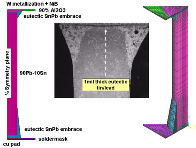
Fig. 7: Conventional CGA Geometry Definition
